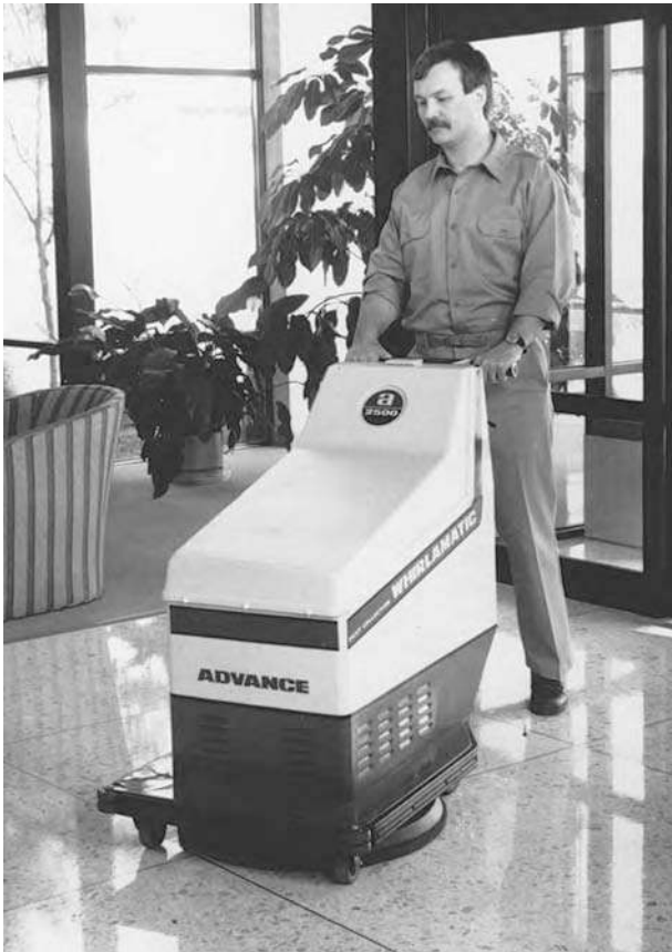
Figure 5-10 Burnishing a terrazzo floor. See also Appendix I. (Used with permission of the Advance Machine Company.)
