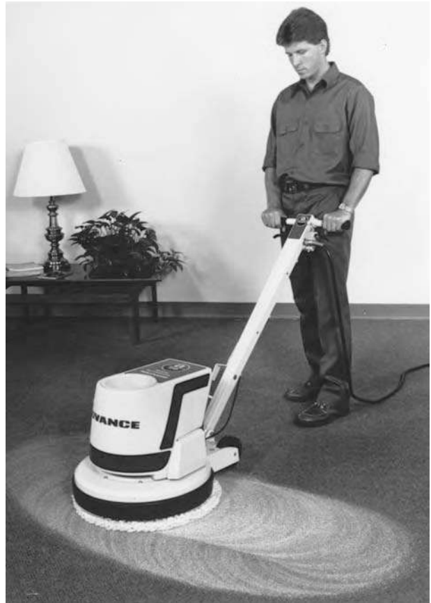
Figure 5-15 Bonnet cleaning using the “All-Purpose Matador” from Advance. (Used with permission.)
